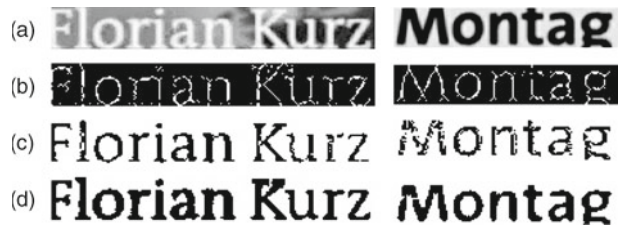
Fig. 9 Seed selection and region growing results: a grayscale image, b skeleton image, c seed image, d region-growing result
