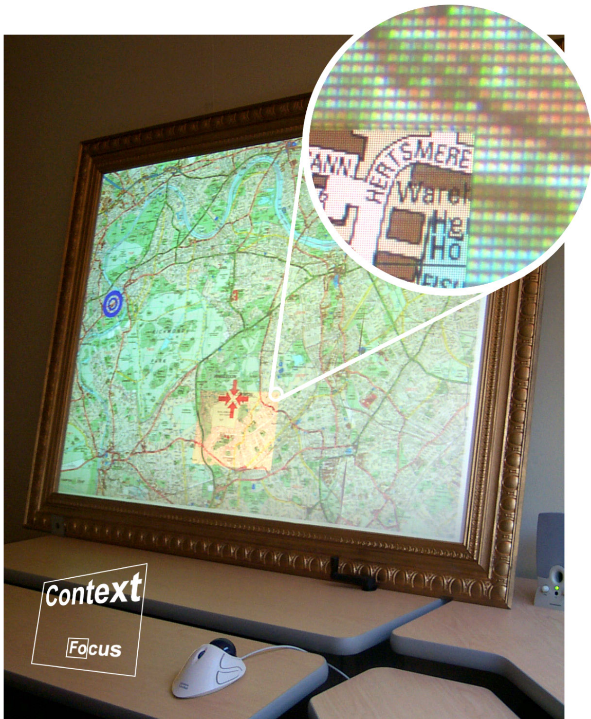
Figure 2.1.: A focus + context interface. The iconic illustration at the bottom left shows where the focus screen is located. The callout shows the different resolutions of focus and context area. Source: [12]
